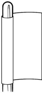
Fig. 16i - Roll the sheet of paper around a broom handle or large diameter dowling.
