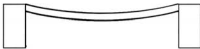
Fig. 37a - How to span a wide gap. Problem: The bridge bends and is weak.
