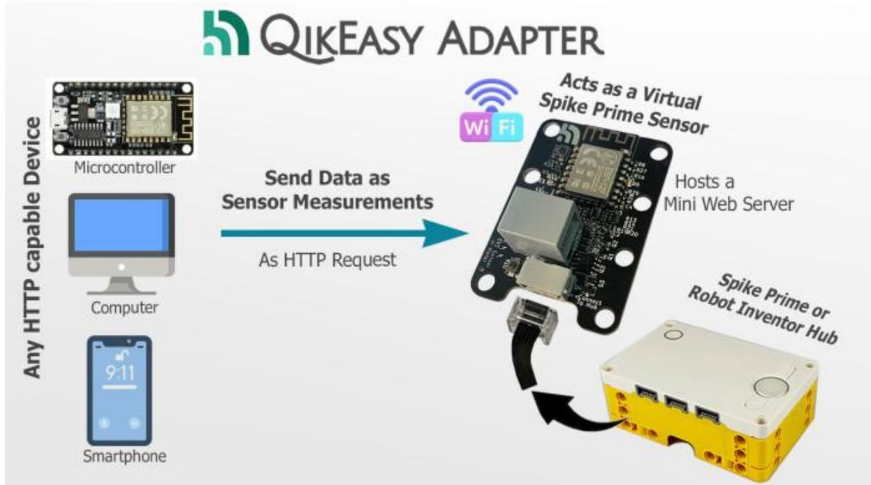
The following demo illustrates the power of adding wireless capability to your Spike Prime or Robot Inventor system. As a bonus, we also show you how you can use Amazon ALEXA voice commands to activate actions on your LEGO robot. Using IFTTT, one will be able to enable Google Assistant and other triggers in the same way.
